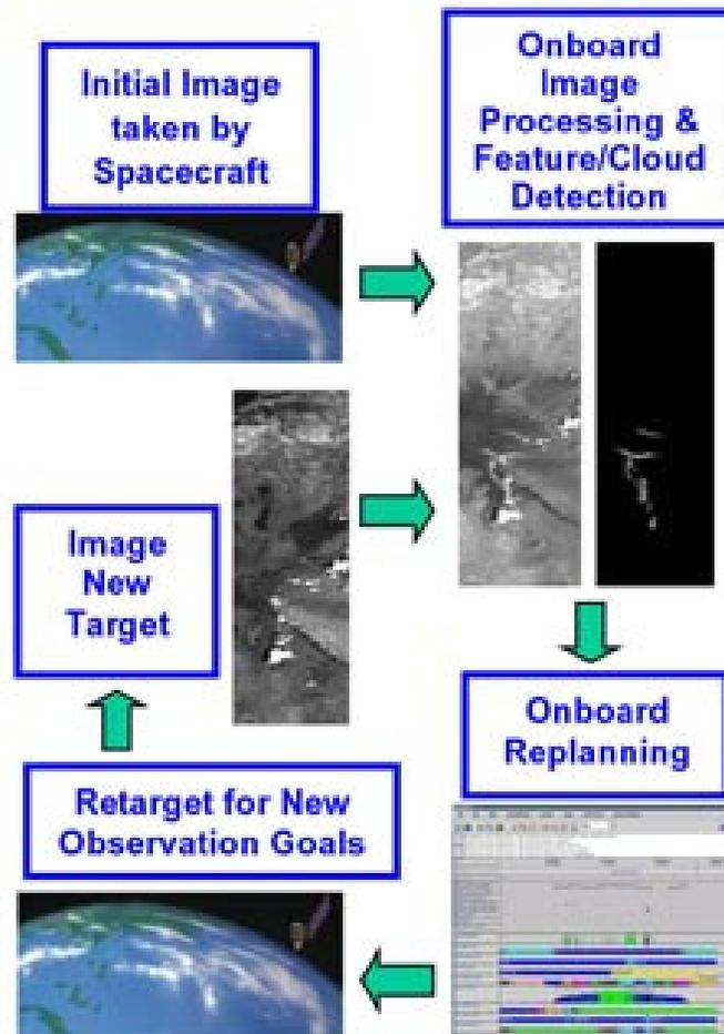
***Just as changing cloud patterns on Earth were identified using Earth Observing-1's Advanced Land Imager along with ScienceCraft software, the THEMIS instrument with ScienceCraft on the Mars Odyssey spacecraft can avoid transmitting useless images.***
